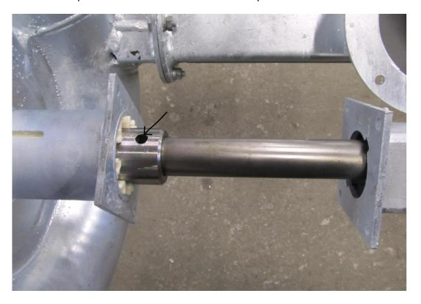
Remove the cutter from the pump housing and pull the impeller out of the pump housing.
