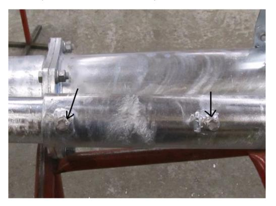
Release four screws that secure the cover tube to the pump housing.
