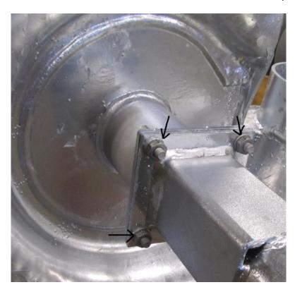
Loosen the cover from the pump housing and push it up to expose the shaft. Push out the pin which secures the shaft to the impeller.
